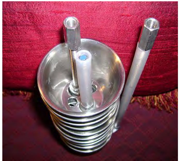
Again using the tubing to protect the rod, ensuring that the electron will travel through the stack and not bypass any cups causing current leak.
