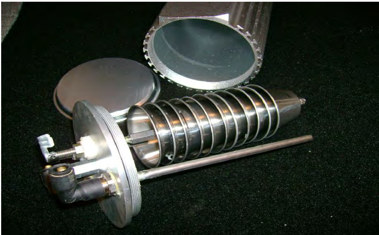
Single cell mounted in extruded aluminum container. Legris fittings, and the clip taken from spark plug wires that attach the the plug, snaps right on the 1/4x20 threads.
