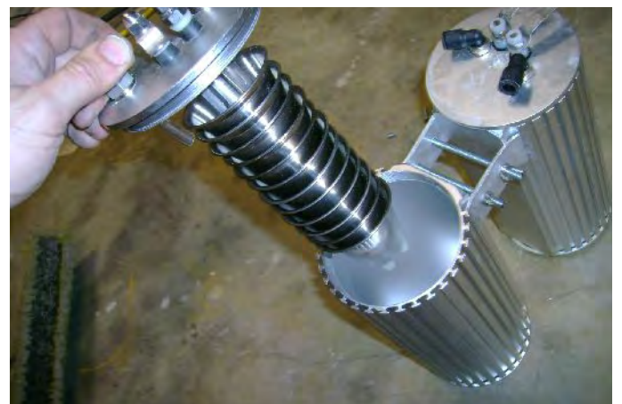
Electrode mounted in an extruded heatsynk outer container with screw on top and bottom. Legre or swag- lock fittings were used
