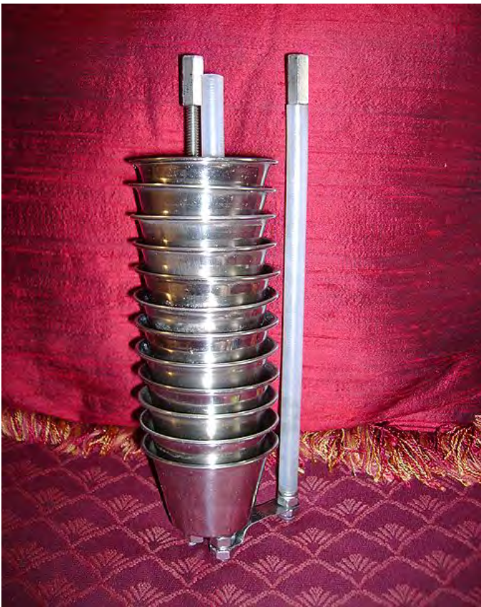
The TwisterHHO Electrode set up for top connection Notice the Teflon tube covering the connection rod. This is to ensure the current would not bypass the cell and jump from the rod to the cups.
