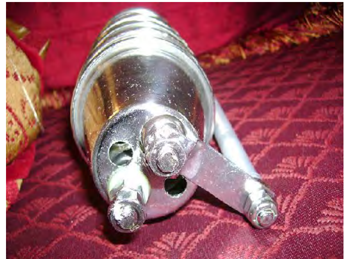
Bottom of the electrode showing the flattened u clamp used to connect each of the cups properly in parallel
