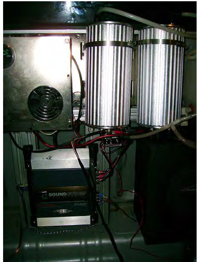
2000 Ford F-150 V8 This rig is mounted where the back seat was originally. It included a video camera (the silver looking thing pointing at the bubbler) viewing the production through bubbler that ran video to my 7" flip out screen on the stereo head unit. The purple container is an overflow container. The cell was controlled by a potentiometer that was mounted in the center console that controlled a 12-24v Kelly controls pwm.
