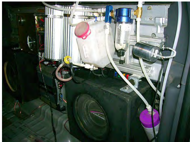
2000 Ford F-150 V8 This rig is mounted where the back seat was originally. It included a video camera (the silver looking thing pointing at the bubbler) viewing the production through bubbler that ran video to my 7" flip out screen on the stereo head unit. The purple container is an overflow container. The cell was controlled by a potentiometer that was mounted in the center console that controlled a 12-24v Kelly controls pwm.
