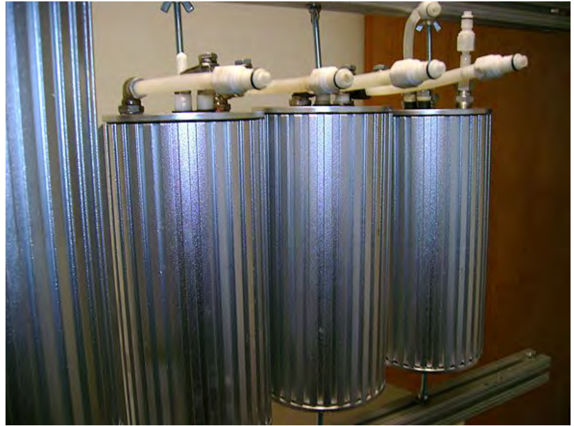
Three Cell Testing unit, mounted in 80/20 aluminum rack. This setup is what I would use to do ltr/min testing on different power supplies and circuits. TO the left side are two stacked cells, the top was the bubbler and the bottom acted as a reservoir with pressure gauge mounted in the top.
